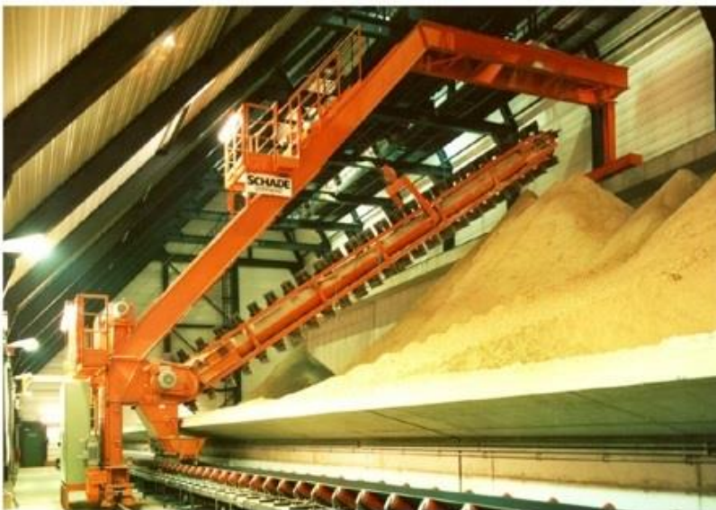
Semi-Portal Scraper Reclaimer
