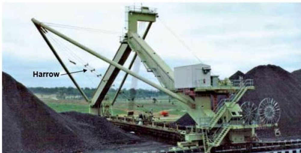
Portal Bridge Reclaimer
