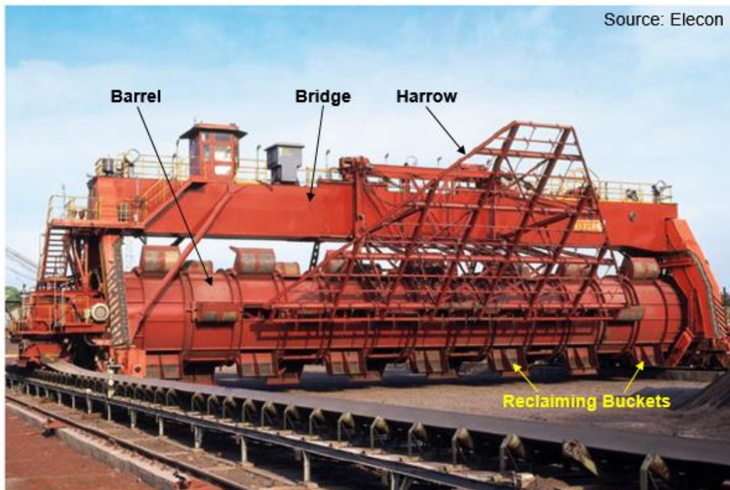
Barrel Type Reclaimer
