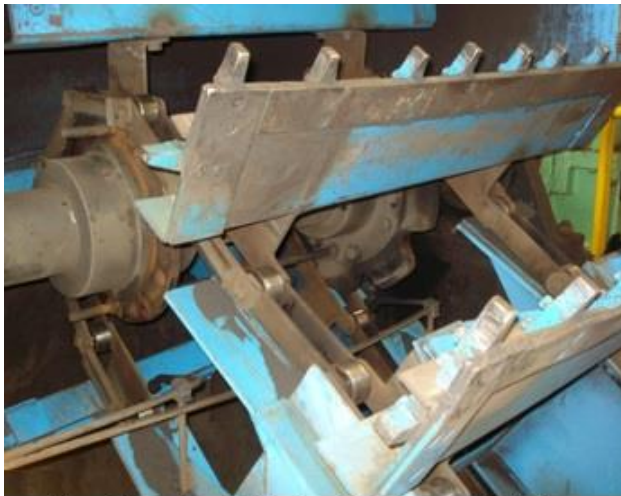
Two Strands of Chain with Scraper Blades
