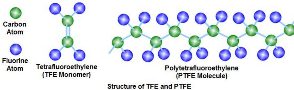
The fluorine atoms covering the carbon chain protect it from chemical activity. They also repel other PTFE molecules and molecules of other substances resulting in high chemical resistance and exceptional non-sticking properties of polytetrafluoroethylene.
