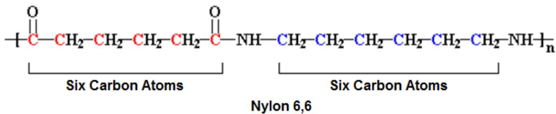
The nylon structure shown in above figure is called **nylon 6,6** because each repeat unit of the polymer chain has two stretches of carbon atoms, each being six carbon atoms long. The polymer is made by reaction between adipic acid and hexamethylene diamine.
