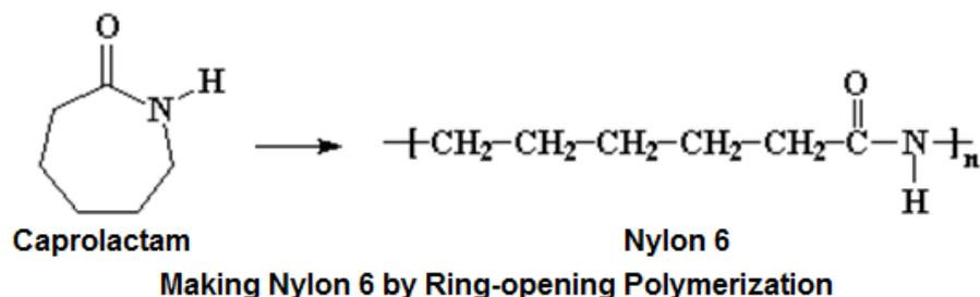
It is called nylon 6 because each repeat unit of the polymer chain has only one kind of carbon chain, six carbon atoms long.
