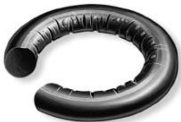
Failure Due to Hardening
