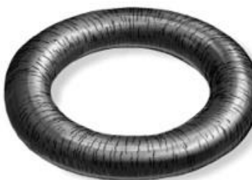
Weather and Ozone Cracking
