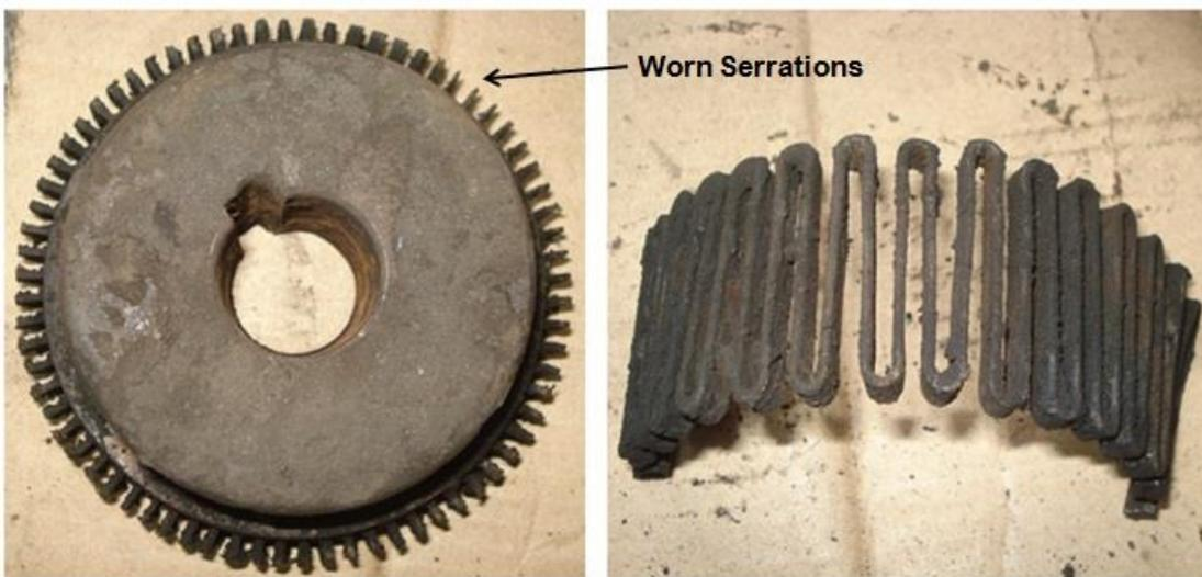
**Wear of Grid Coupling Serrations Due to Loss of Lubrication**
