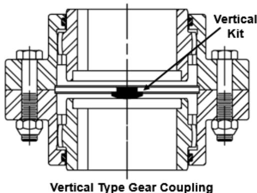
As shown in above figure, gear couplings designed for use with vertical shafts consist of a vertical kit which keeps the sleeve in the designed position.
