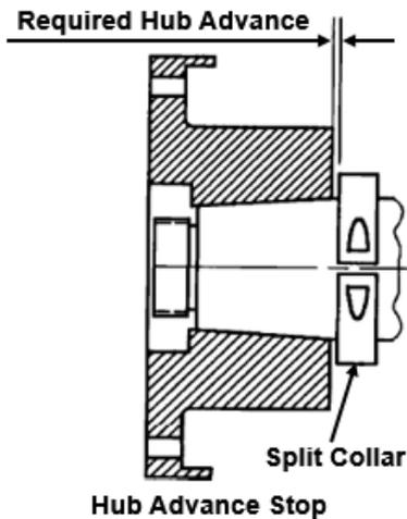
Above figure shows a stop in place, in the form of a split collar secured to the shaft, to limit the tapered hub during its advance up the taper. The coupling nut should immediately be placed on the shaft after hub installation to prevent the hub from "walking down the shaft." When the hub cools, it will shrink to some amount in the length direction. The coupling nut should then be tightened again.
