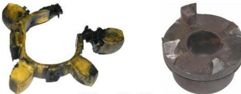
**Spider and Hub Failures**
