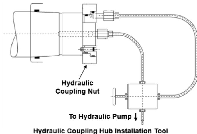
Above figures show a keyless hydraulically dilated coupling shaft and the hydraulic coupling hub installation tool. For installing the coupling, a hydraulic pump is used to pressurize inside
