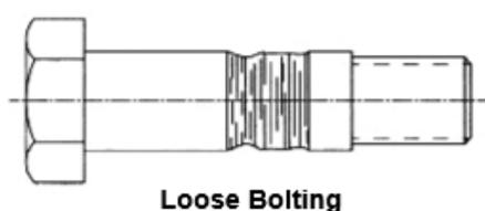
Above figure shows how a coupling bolt would look after loose bolting. Note that the disc has tried to embed in the bolt, causing a reduction in diameter or cutting of the bolt. When this failure occurs, the bolts and disc pack should be replaced. Torque should be applied to the nut and not the bolt.
