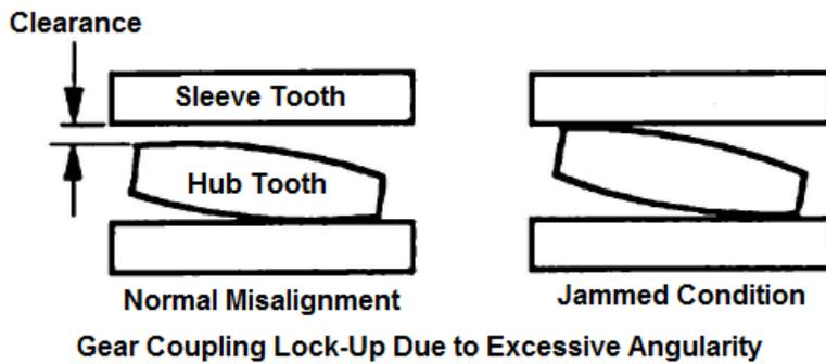
Fretting occurs when two surfaces move in relation to one another. The loading and heat generated by friction causes metal to be removed, to be transferred, or to crack. Fretting is actually fatigue of metal surfaces. In gear and grid couplings flex members slide in relation to each other. If the heat generated due to sliding exceeds the lubricant's ability to perform its function, major fretting occurs.
