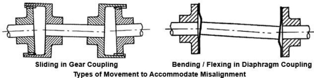
**Sliding in Gear Coupling**
