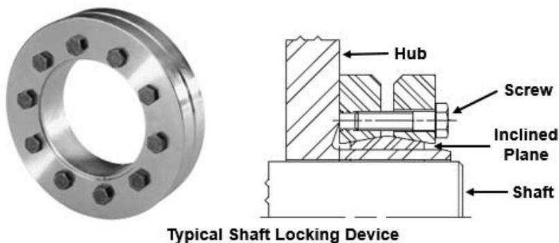
The contact pressures created using a shaft locking device can be greater than traditional interference fit pressures, allowing for more torque to be transmitted or shorter hubs to be used. The easy installation also allows the hub to be positioned more accurately on the shaft.
