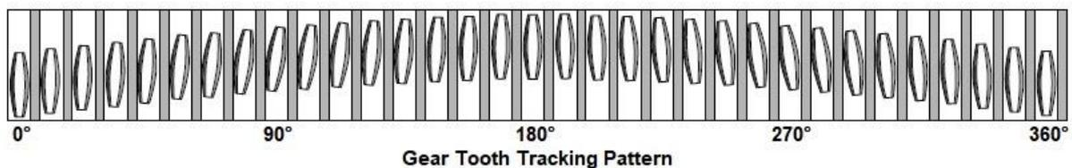
Above figure shows gear tooth tracking pattern (through  $360^\circ$  rotation) when subjected to misalignment condition.
