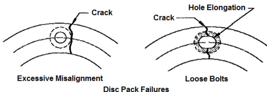
Above figure shows disc pack failure due to excessive misalignment and loose bolts. Due to excessive misalignment, cracks usually start on the outer discs and progress inward. If hole elongation and cracking is found, it is most likely due to loose bolting.
