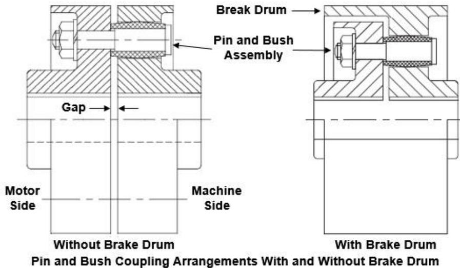
The coupling can be fitted with add-on parts such as brake disk or brake drum. Above figure shows typical coupling arrangements with and without brake drum. As shown in above figure, many coupling manufacturers provide guard on nuts for safety. Recommended amount of gap between coupling hubs is very important to compensate for shaft misalignment.
