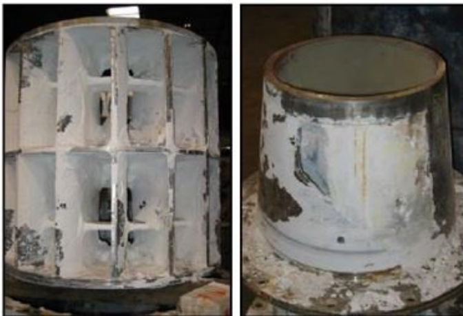
Calcium Coated Rotor and Cone
