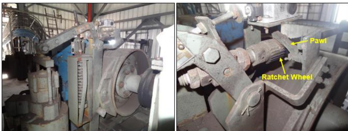
Automatic Recovery Device Utilizing Pawl and Ratchet Wheel
