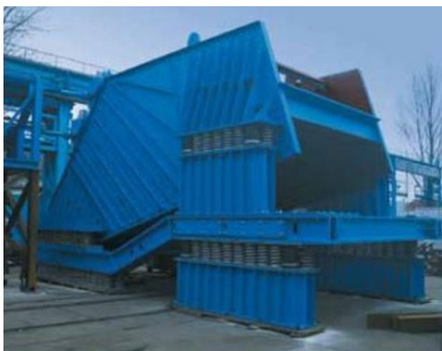
Vibrating Screen with Sub-frame
