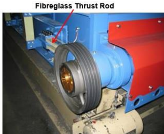
Transfer of Motion to Outer Frame
