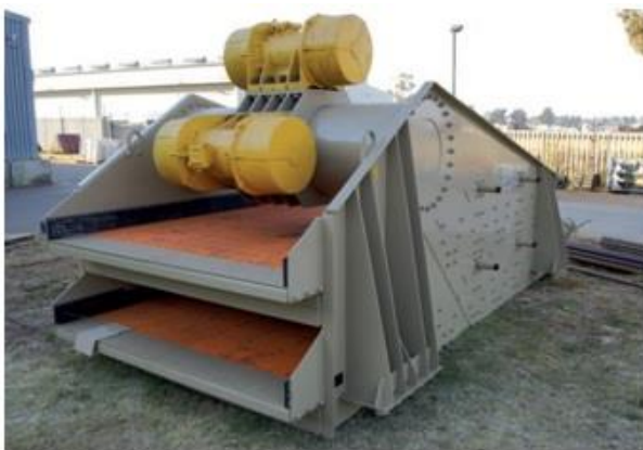
Screen Operated by Two Unbalance Motors
