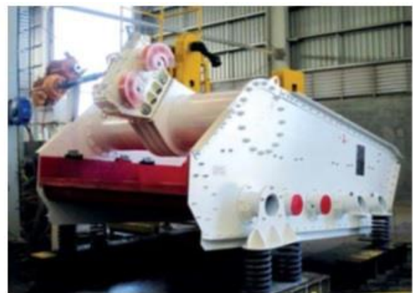
Screen Operated by Unbalance Exciter
