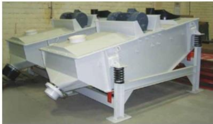
Screen with Single Unbalance Motor
