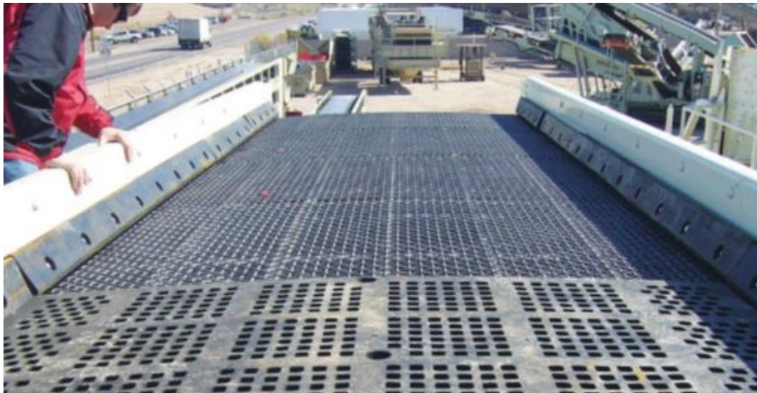
Rubber and Wire Cloth Screen Deck with Rubber Lined Tension Plates
