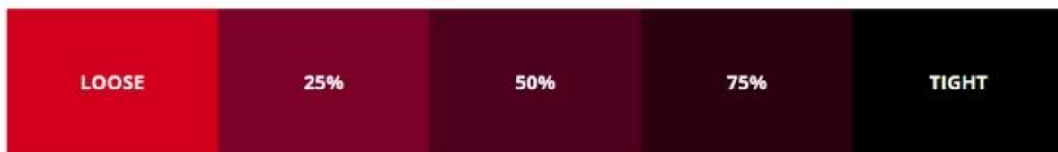
Color Changes Showing Bolt Stretch
