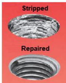
Repair of Stripped Threads
