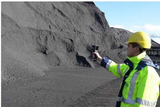
Use of Handheld Camera for Monitoring of Coal Stockpile
