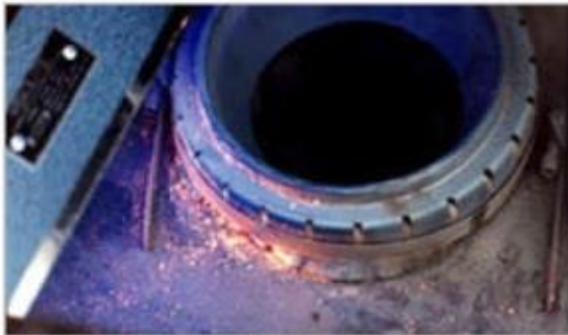
Visolite Glow Reveals Air Leaks
