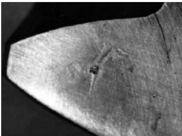
Bending Fatigue Crack
