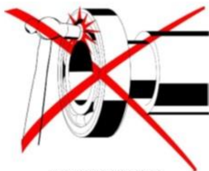
No Hammer Blows
